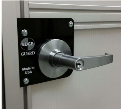
Standard Lever Style Lock – Supplied with our doors. Keyed on the outside pushbutton inside. Normally they are used with a classroom function but can be changed to storeroom.
